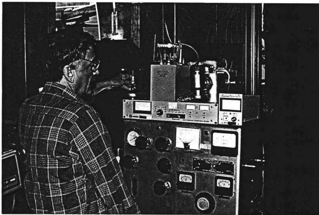
Ron Kovac pulling vacuum on a quartz sample tube
